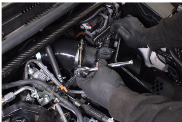
23. Tighten the jubilee clip securing the silicone to the intake pipe.
