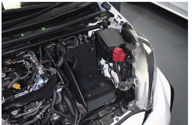
26. You do not need to fully secure the air box. You need some movement to install the intake pipe.
