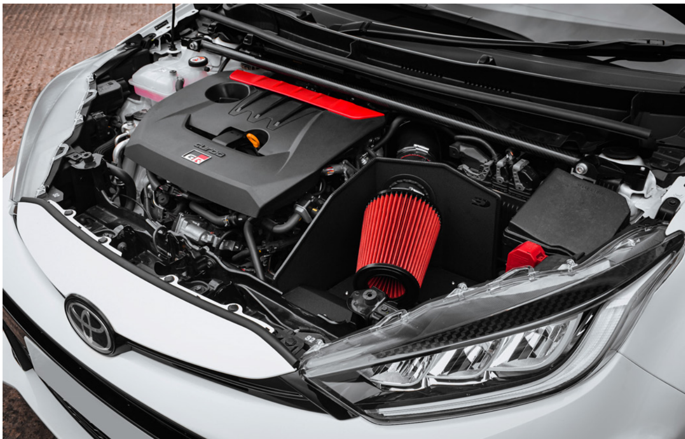
20. The Direnza Cold Air Kit is now installed.
