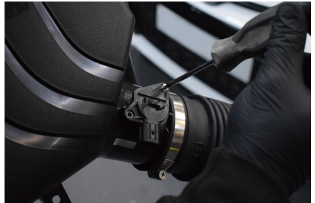
18. Remove 2x screws securing the MAF sensor using a philips screwdriver..
