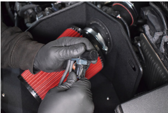
21. Plug in the boost control solenoid.
