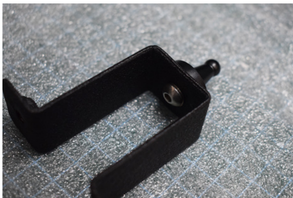
24. The third mounting bobbin is installed onto the 'U' shap bracket.
