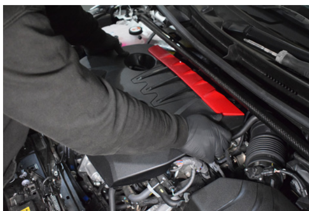
4. Pull off the engine cover to give you access to the throttle body jubilee clip.
