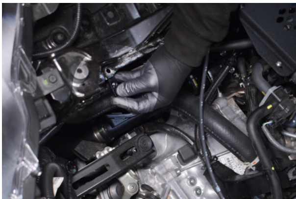
27. Install spire clip onto the front panel of the car.
