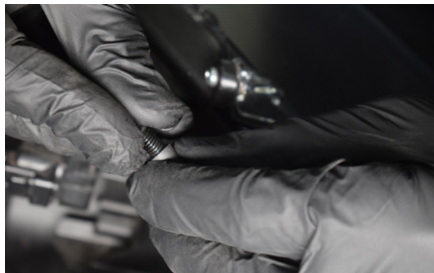
22. Blank off the vacuum pipe by inserting a bolt, ensure it is a tight fit.
