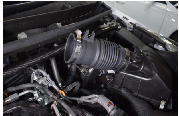
14. Release the intake piipe from the throttle body and pull away entire airbox assembly to remove.
