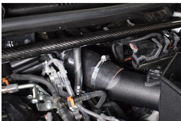
21. Place 2x jubilee clips over the silicone joiner, before pushing the intake pipe into the silicone.
