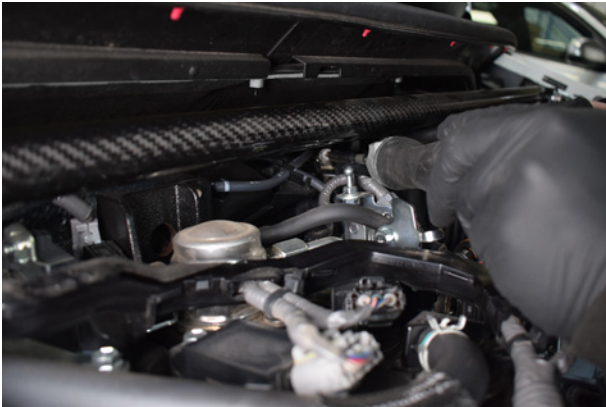
13. Undo the jubilee clip securing the intake pipe to the throttle body.
