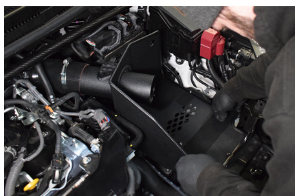
22. With everything in place, you can push down on the heat shield to fix bobbins into place.
