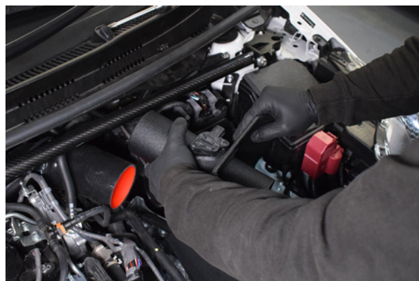
20. Slide the intake pipe into the hole in the heat shield.
