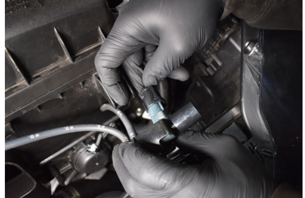
8. Unplug the boost control solenoid.
