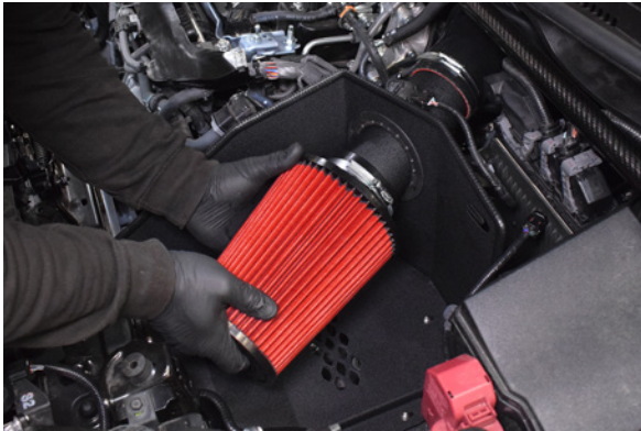
19. Install the air filter onto the intake pipe.
