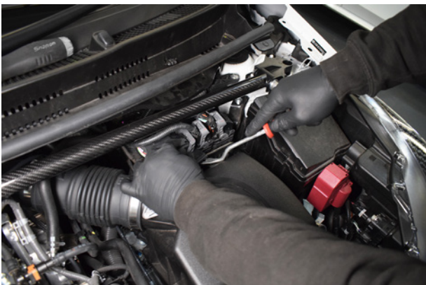
11. Use a trim tool to remove the 2x mounting tabs holding the MAF sensor wiring.
