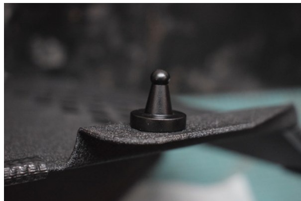
20. Install the 2x bobbins into the pre drilled holes on the heat shield.
