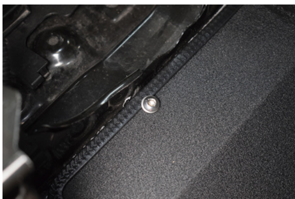
23. Secure the front of the heat shield by using supplied screw into the spire clip you installed earlier.
