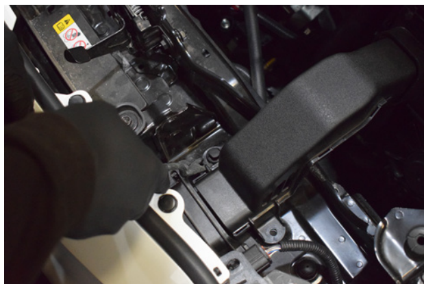
2. Remove 2x clips on the air scoop using a trim tool.
