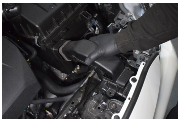
3. Once the clips have been taken out you can remove the scoop.
