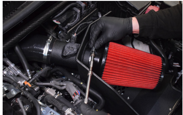
20. Tighten the jubilee clip on the air filter.
