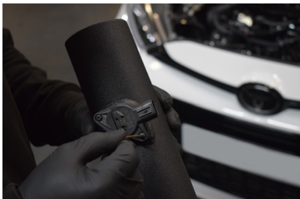
19. Install the MAF sensor into the Direnza intake pipe.
