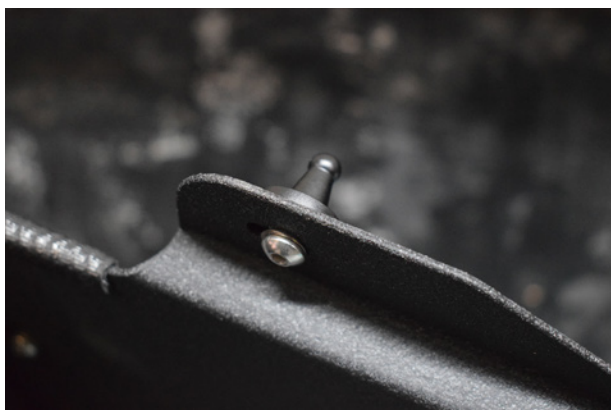
21. Secure the bobbins using supplied screws.
