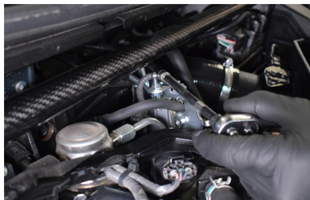
24. Tighten the jubilee clip securing the silicone to the throttle body.
