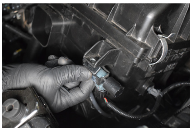
6. Undo screw and release the boost control solenoid from the Airbox bracket.
