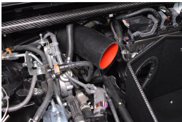
19. Install the silicone onto the throttle body.
