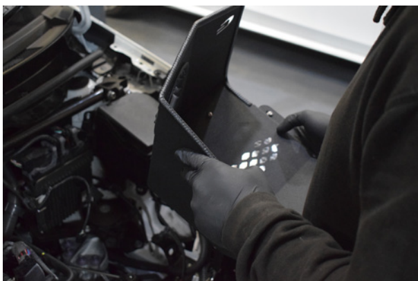
25. The heat shield can now be positioned into the engine bay.
