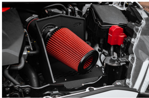
20. The Direnza Cold Air Kit is now installed.
