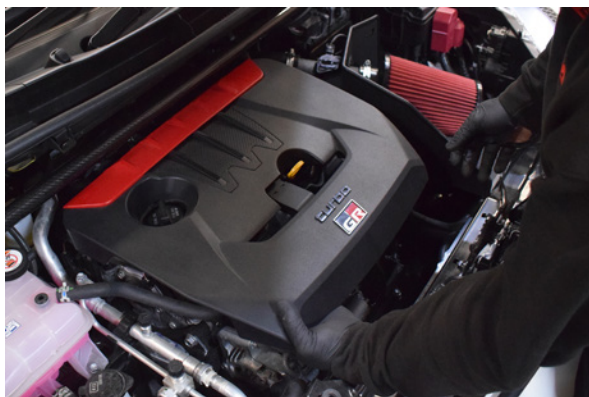
19. Re-install the engine cover.
