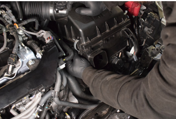
9. The solenoid is clipped into the side of the airbox, remove from clip.
