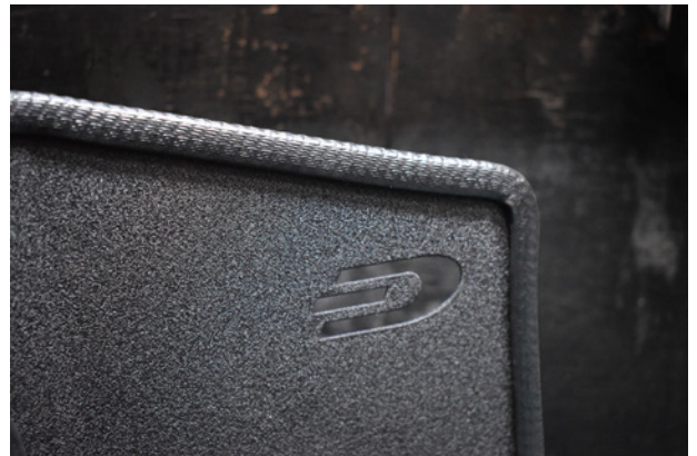
16. Install the supplied edging trim around the edge of the heat shield.
