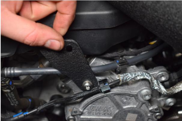
19. Before lowering the intake pipe into position, install the lower bolt of the intake pipe bracket.
