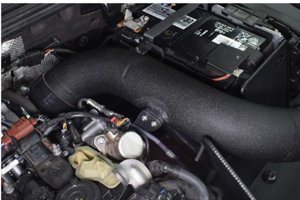
23. Install supplied bolts and washers to secure the bracket to the intake pipe.
