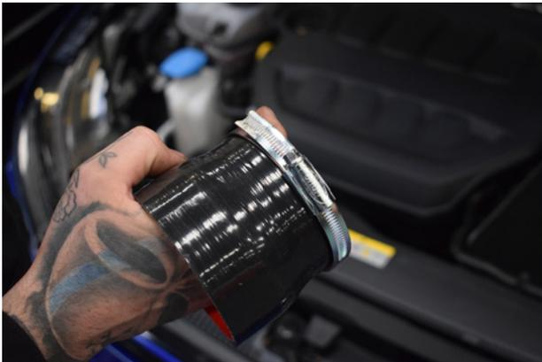
27. Place jubilee onto silicone reducer and place onto the throttle body.
