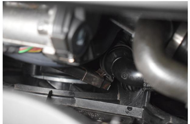
10. Using a spring clip tool, undo the clip securing the recirculation pipe to the recirc valve.
