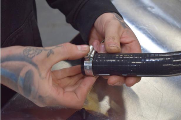
13. Place a jubilee clip on each end of the silicone recirculation pipe supplied in the kit.
