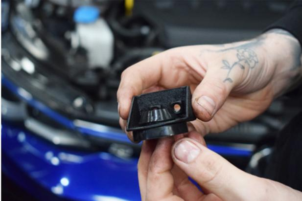
19. The third bobbin is installed on the Airbox support bracket.
