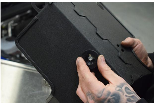
17. Install 2x Polyurethane bushes into the Airbox.
