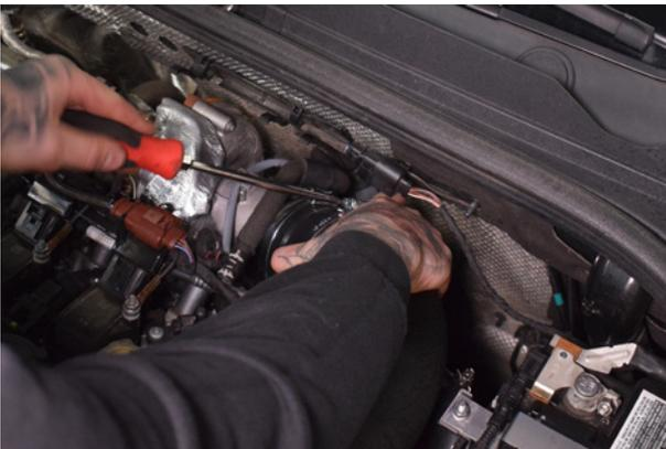
21. Using a flathead screwdriver, tighten the 2x jubilee clips on the silicone reducer.
