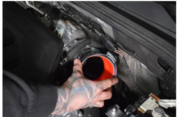
28. Place another jubilee clip onto the silicone reducer before installing the intake pipe.
