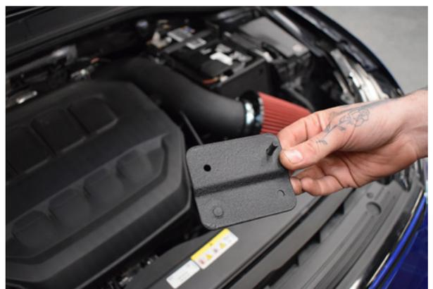
24. This relocation bracket is need as the intake pipe is now larger and can foul against the sensor.
