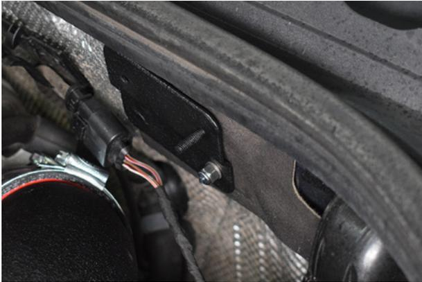
19. Install bracket on OEM stud and secure using supplied nut.
