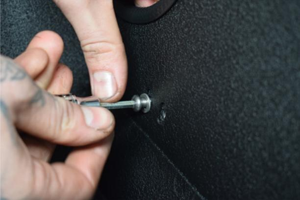
25. Fasten the Airbox to the Airbox bracket using 2x supplied bolts and washers
