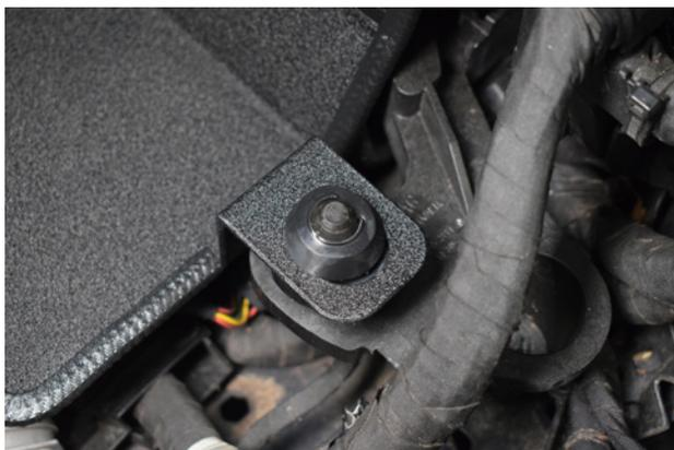
23. Ensure the bobbins are securely mounted on the OEM mounting points.
