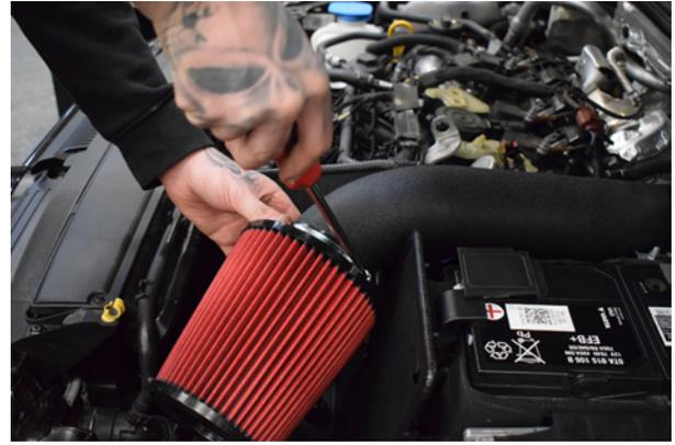
20. Tighten the Air Filter jubilee clip using a flathead screwdriver
