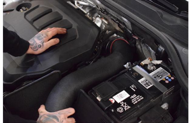
20. You can now slide the intake pipe into the silicone reducer and lower into the correct position.
