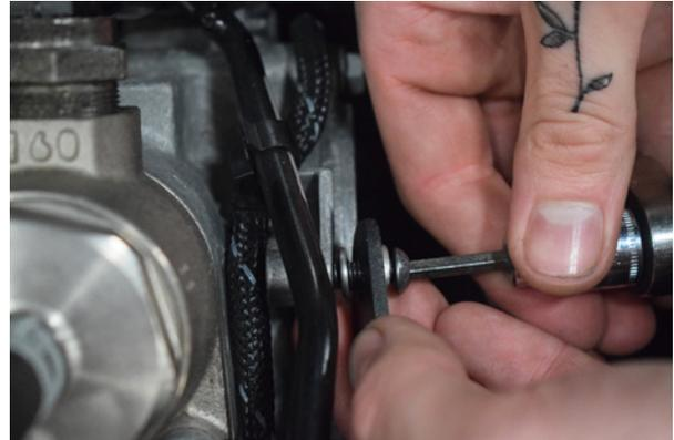
16. Loosely fix the bracket into position.
