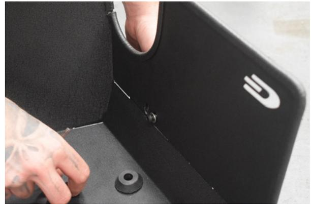
10. Install and tighten supplied bolts to fix the bracket/bobbin to the airbox.
