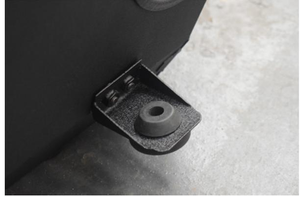
8. Install the bobbin into the bracket and install on the Direnza air box.
