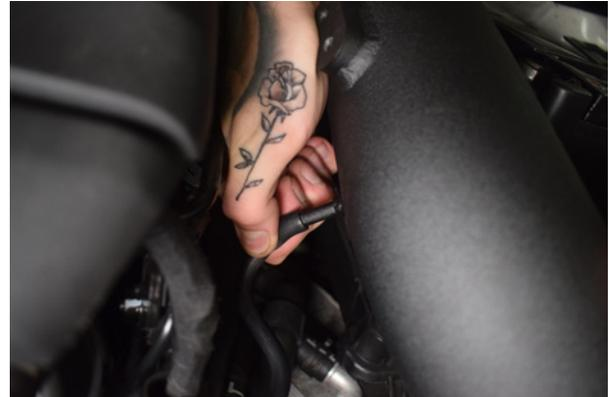
20. Install the breather pipe on to the new hard pipe.
