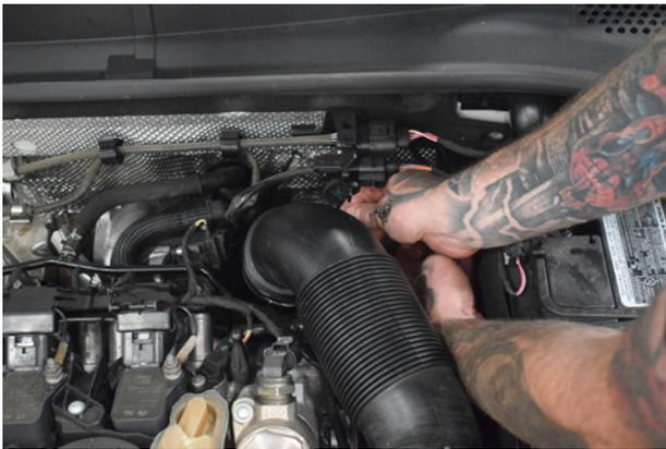
3. Undo jubilee clip on the OEM throttle body intake pipe.
