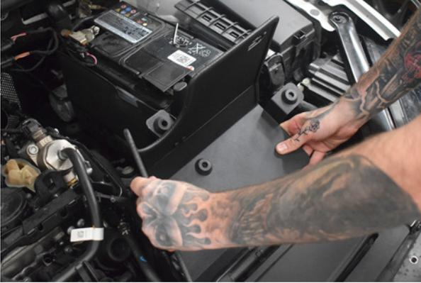
13. Install the edging trim before placing the airbox into position.
