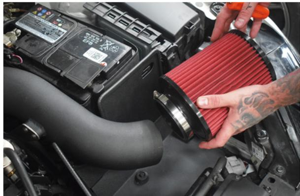
24. Place filter onto the opposite end of the hard pipe.
