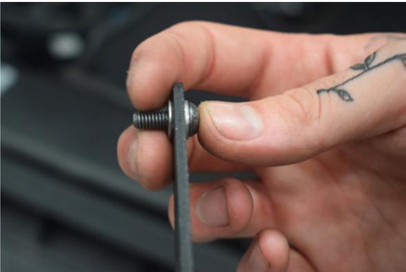
15. When installing the hard pipe support bracket, ensure the washers are positioned like this.
