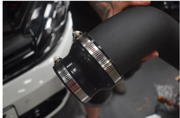
18. Install the silicone reducer and 2x jubilee clips on the throttle body end of the hard pipe.
