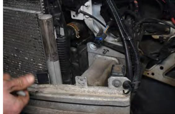
86. Secure using 6x 16mm bolts, (three per side).
