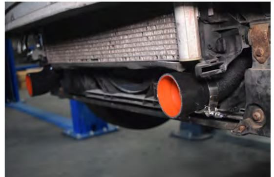
94. Place 2x clips onto the end of the hardpipes.
