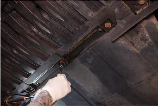
1. Remove 7x 10mm bolts from the engine under tray.
