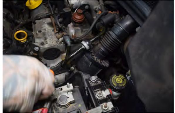
50. Undo the jubilee securing the cold side boost pipe to the sound enhancer unit.
