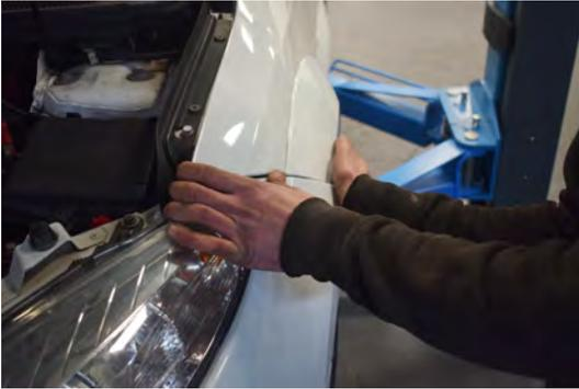
127. Push in the sides of the bumper once fitted in position.
