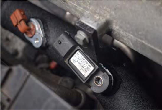
67. Fit the pressure sensor into the cold side hard pipe.
