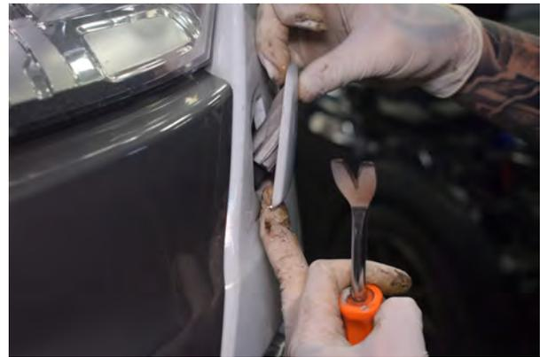
10. Remove the washer jet by pulling out the mechanism and rolling off plastic cover.
