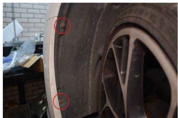
6. Under the wheel arch, remove 2x T20 torx, do this on both sides.
