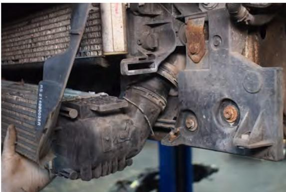
47. Pull away the intercooler from the boost pipes.
