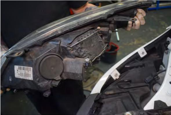
13. Lift and remove headlight, remembering to unplug all connections.
