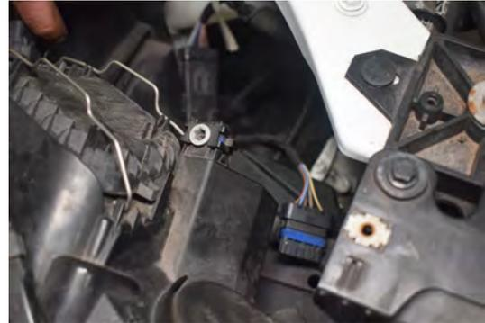
122. Re-install 2x headlight connections and place into position.
