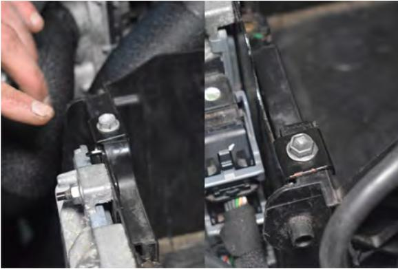
31. Undo 2x 10mm bolts securing the ECU.
