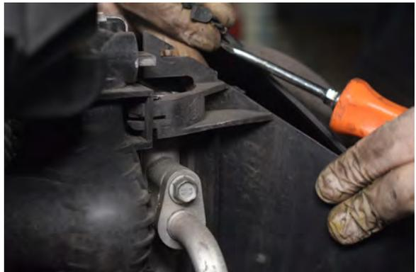
54. Use screwdriver to push clips holding the front cowling.
