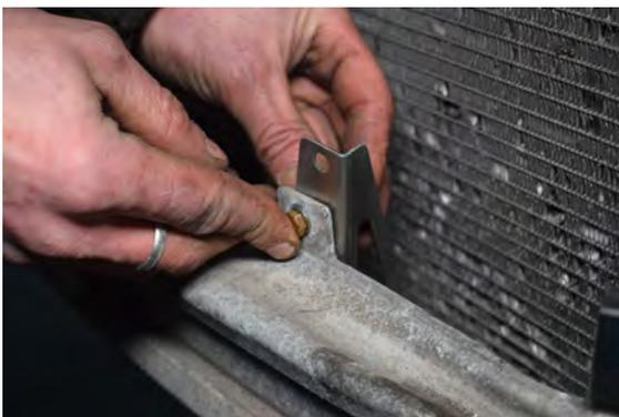
89. Secure the intercooler brackets into position on the lower of the two mounting holes with supplied nuts and bolts.
