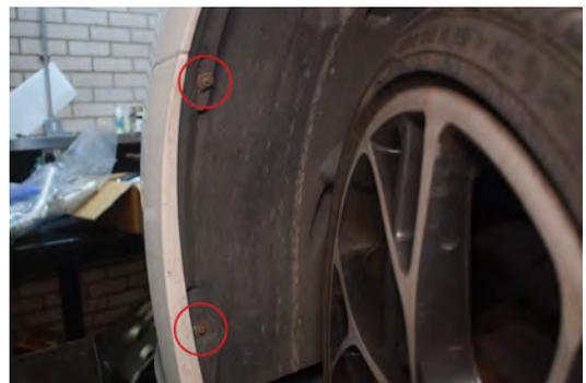
132. Under the wheel arch, install 2x T20 torx, do this on both sides.
