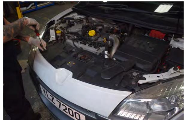
4. Remove 6x T20 torx from the top edge of the front bumper/slam panel.
