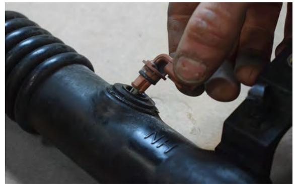
64. Remove sensor from the OEM pipe.
