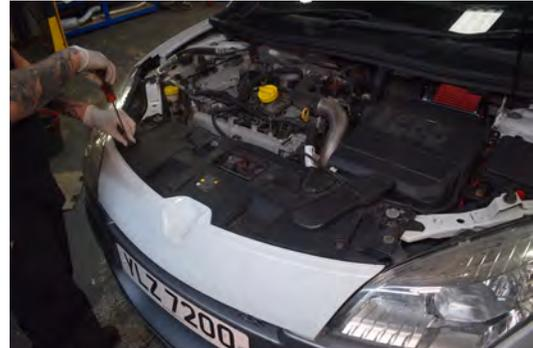
134. Install 6x T20 torx from the top edge of the front bumper /slam panel.
