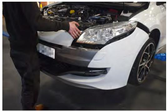
126. You can now begin re-fitting your front bumper remembering to re-connect the washer jet pump and wiring harness.
