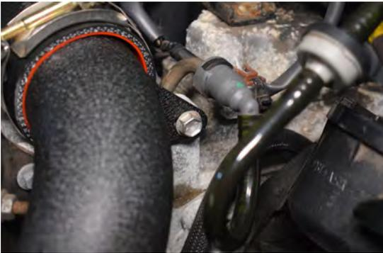
81. Secure with the original 10mm bolt.
