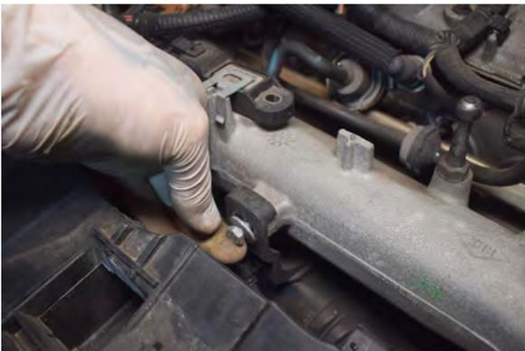
41. Undo the 10mm bolt on the top boost pipe bracket.
