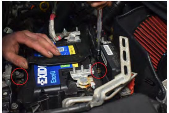
112. Secure the battery with 2x 8mm bolts and battery bracket.
