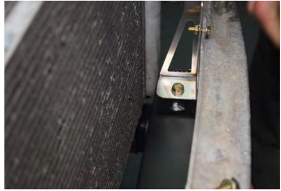
98. Secure the MVT intercooler to the support brackets with supplied bolts.
