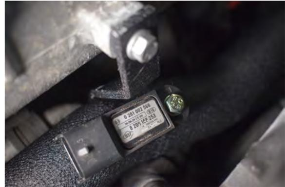
68. Secure sensor with supplied 10mm screw.
