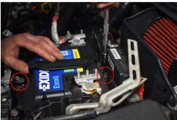
27. Remove 2x 8mm bolts securing battery holder bracket.
