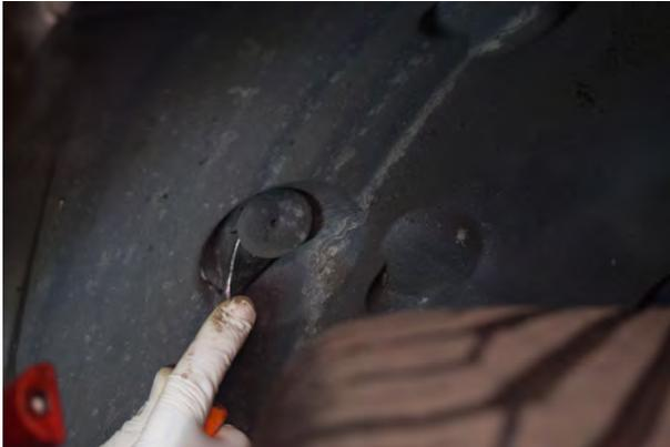
7. Remove 3x push clips under the wheel arch, repeat on both sides.
