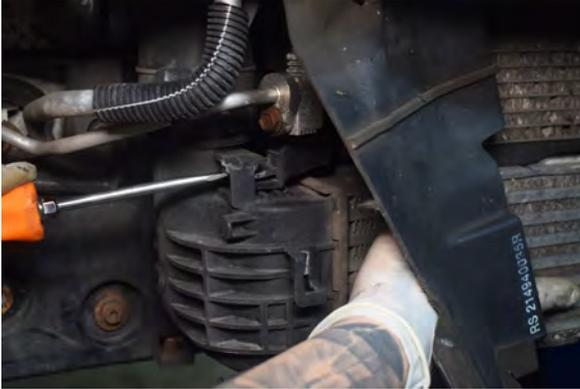
37. Use a screwdriver release the intercooler from mounting point.
