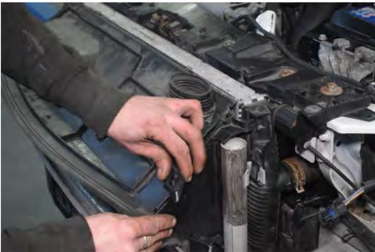
117. Install top ducting with clips.
