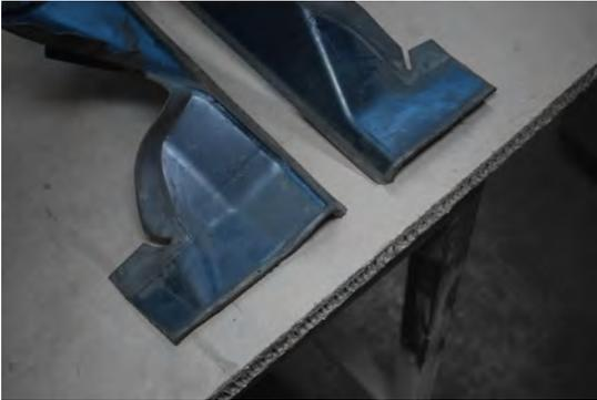
115. The side ducting requires a small amount of trimming to fit around the larger intercooler.
