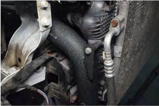
73. Secure 2nd support bracket with supplied 10mm bolt.
