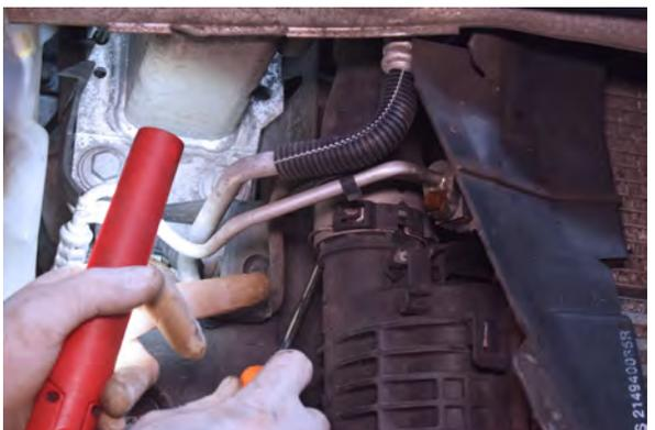
36. Undo the clip on the cold side boost pipe, releasing the intercooler.
