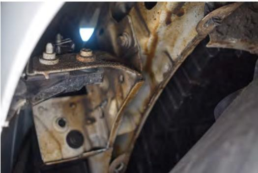
129. Install 3x 10mm screws under the liner and 1x T25 do this on both sides.
