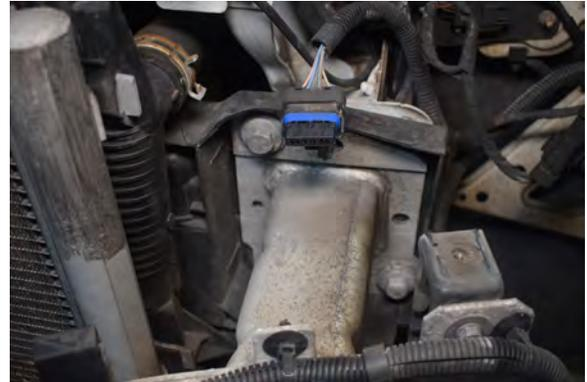
56. Loosen 10mm bolts on the crash, providing access to the cold side boost pipe. You can also remove the crash bar if you wish.
