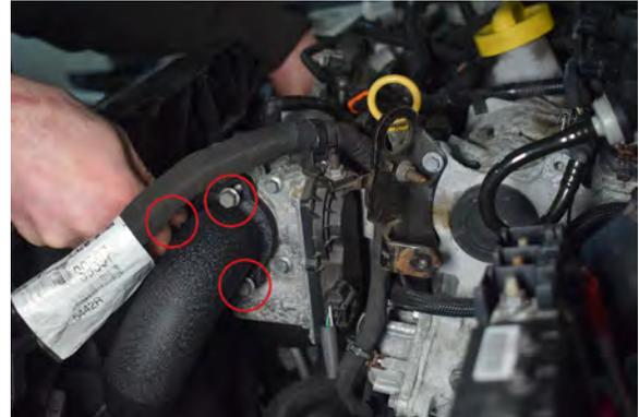
62. Install 3x 10mm bolt securing the new Direnza hard pipe to the throttle body.
