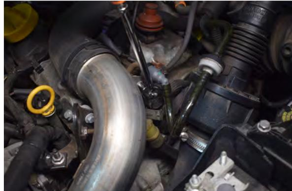
42. Remove 2nd 10mm on the boost pipe bracket.
