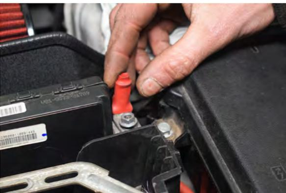
29. Remove 2x 10mm bolts and battery terminal.
