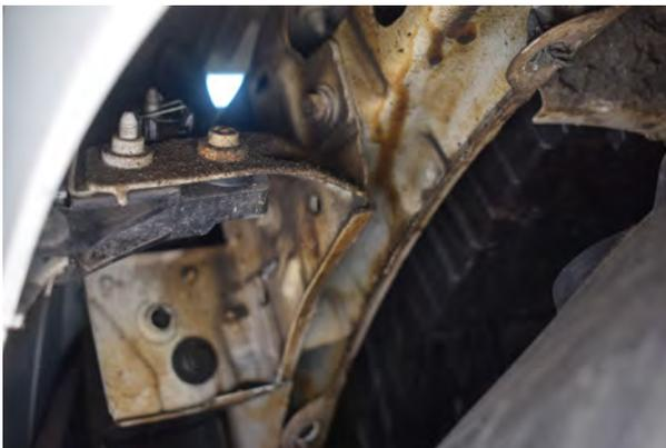
9. Remove 3x 10mm screws under the liner and 1x T25, do this on both sides.
