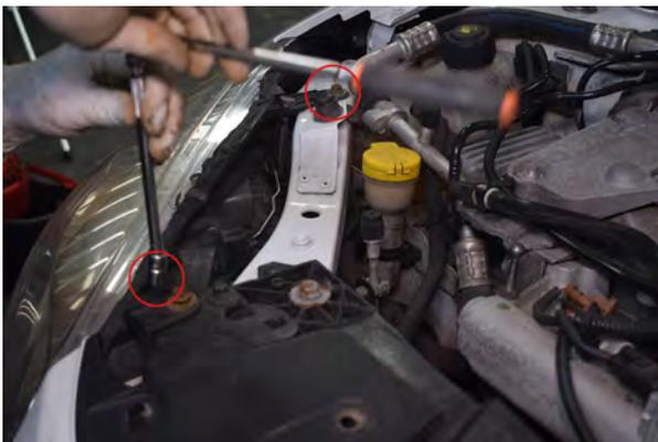
11. Remove 2x 10mm bolts and lift metal clip securing the headlight.
