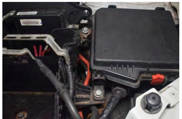
30. Remove 2x 10mm bolts on the cover and remove.
