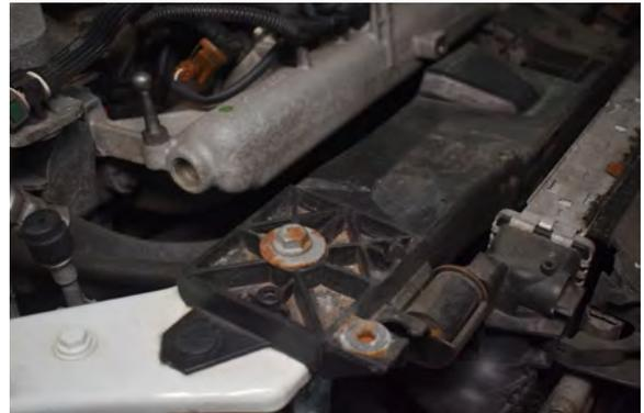
52. Undo 2x 13 bolts on the plastic slam panel.
