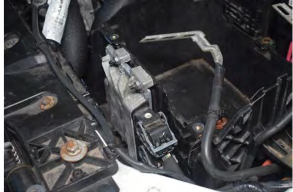
32. Remove ECU and place safely out of the way.
