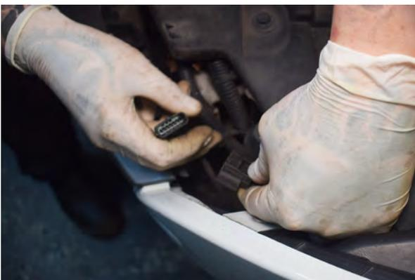
17. Unplug the wiring harness located on the passenger side of the vehicle (RHD drive models).
