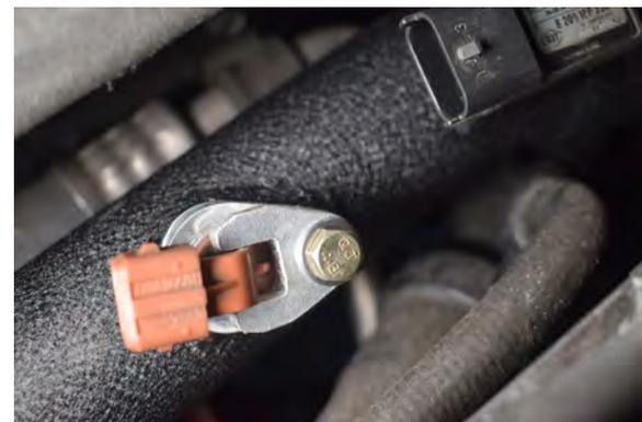
66. Fit the temp sensor and supplied support bracket with supplied 10mm screw.
