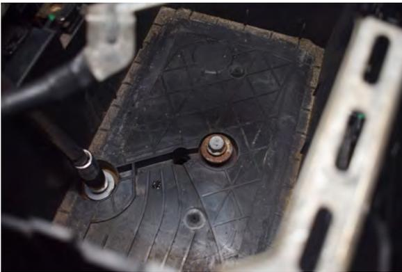
33. Undo 3x 13 bolts holding the battery tray to the car.
