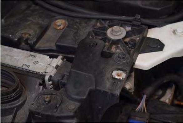
19. Remove 3x 10mm screws from the headlight holder.
