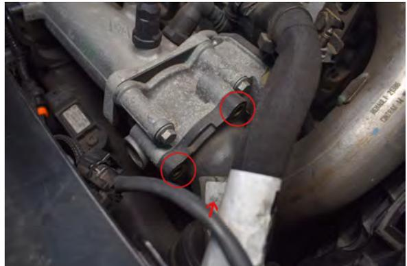
46. Remove 3x 10mm bolts on the throttle body inlet pipe.
