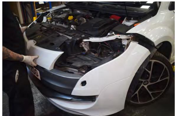
16. Lift and pull the bumper to release.
