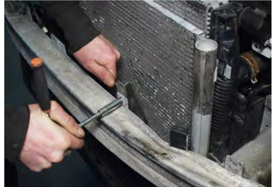
100. You can now tighten all the 10mm bolts securing the intercooler and brackets.
