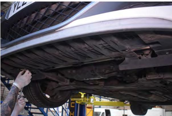
3. Remove 4x 10mm bolts from bumper under tray.
