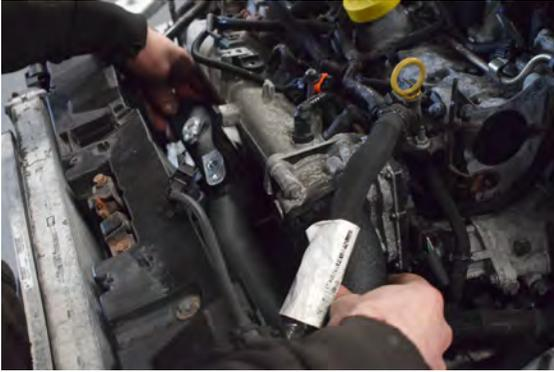
61. Install the first section of the cold side hard pipe onto the throttle body.
