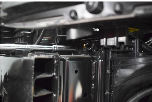
5. Remove the locating nuts on the crash bar, repeat on the other side.
