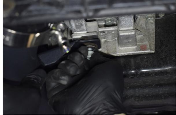
26. Secure the hard pipe using the factory hardware.
