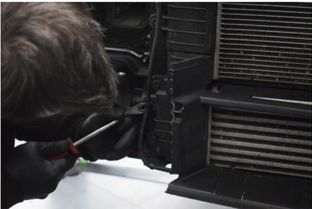
9. Unclip the wiring from the intercooler shroud.
