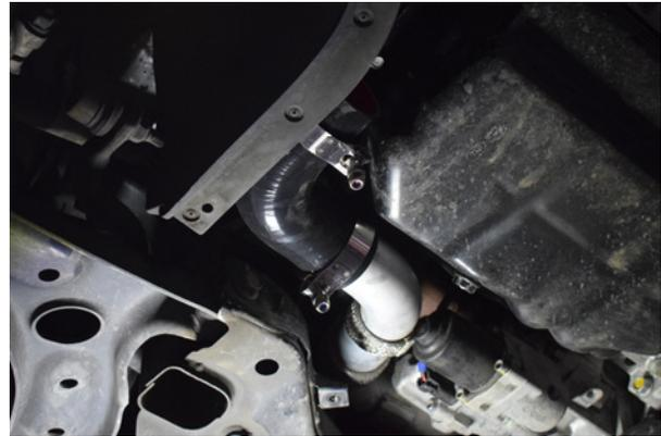
20. Install the 90° silicone jointer onto the alloy hard pipe along with two supplied clamps.
