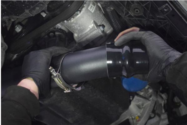
25. Install the straight silicone joiner onto the end of the hard pipe.
