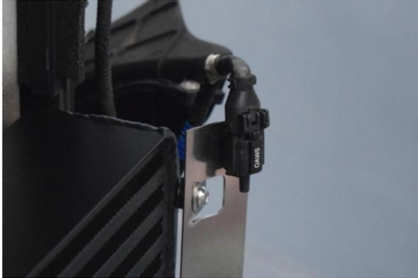
37. The sensor can be clipped into the keyhole slot on the shroud.
