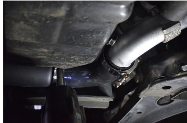
28. Nip up all clamps to hold the pipework together while allowing some movement.
