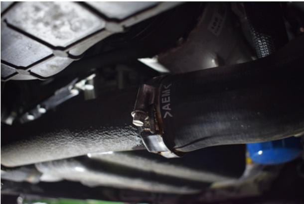
3. Undo the hose clamp that secures the rubber pipe to the hard pipe on the hot side of the intercooler.
