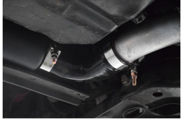
38. You can now fully tighten all hardware and clamps on the intercooler pipework.
