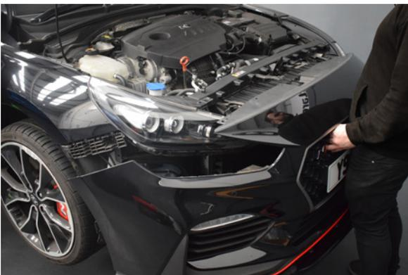
45. Install the front bumper remembering to connect the bumper loom on both sides.
