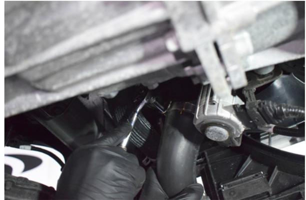
16. Remove the clamp securing the boost pipe to the throttle body.
