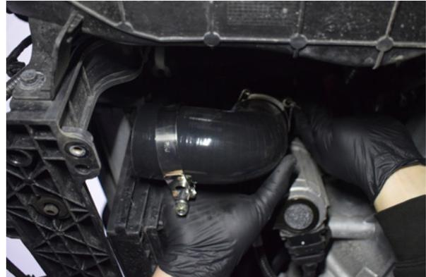
32. The second 90° silicone can be installed, this will be the join between the throttle body and MVT.
