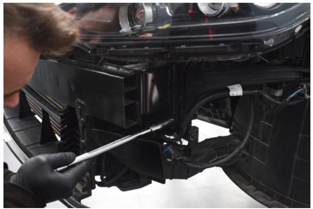
6. Remove 4x bolts securing the crash bar, repeat on the other side.
