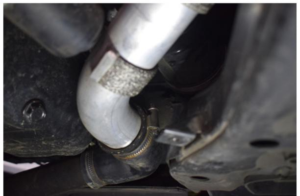
18. On the other side, remove the clamp located on the silicone positioned between the two hard pipes.
