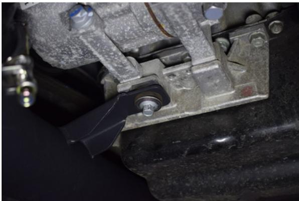
27. Don't fully tighten just yet, this will allow some movement when installing the intercooler.
