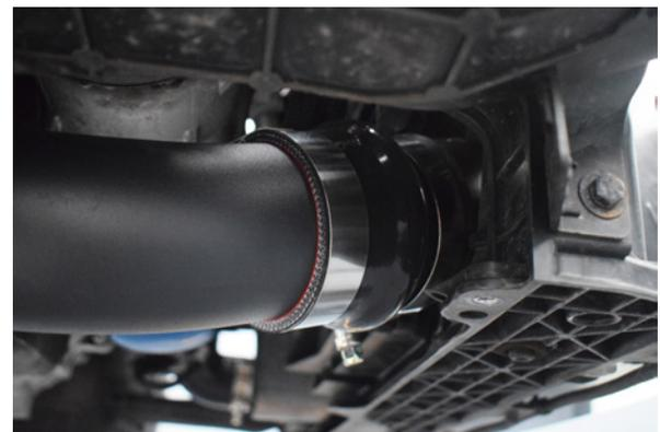
36. With the intercooler secured, you should be able to manipulate the silicone hoses over the intercooler inlet/outlet on both sides.
