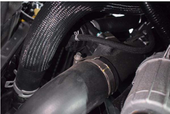
15. You can now begin removing the remaining factory boost pipes that get replaced as part of the MVT Kit.
