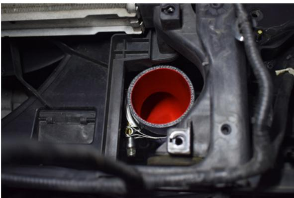
33. Place all clamps over the silicone hose in preparation for installing the intercooler.
