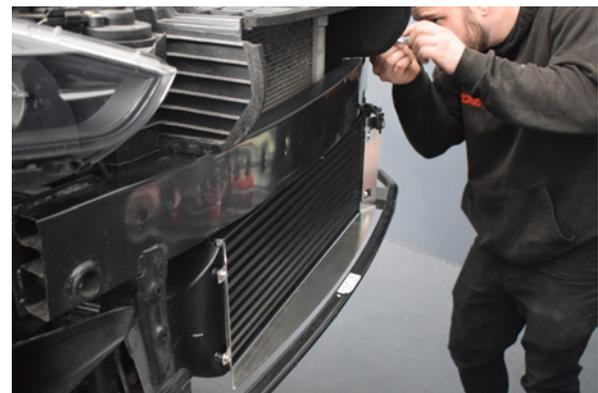
42. It will sit on the locating studs, secure the nuts on these studs first.
