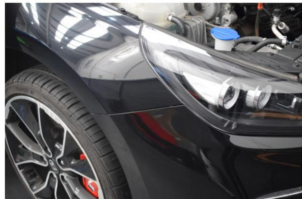
46. The edges of the bumper will clip into position, re insert plastic clips in the wheel arch liner.
