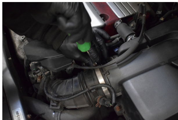
2. Undo the jubilee securing the intake pipe to the airbox.
