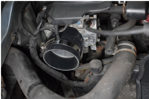
27. Place the silicone joiner on the throttle body with one of the supplied jubilee clips.
