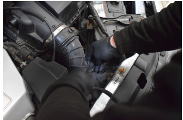
14. Remove heater hose from the clip on the side of the intake pipe..
