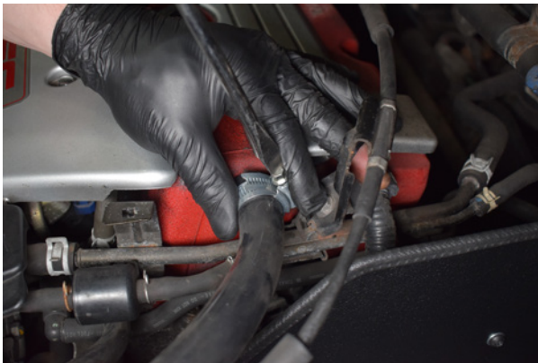
40. You can now install the larger breather pipe, following the same steps as above.
