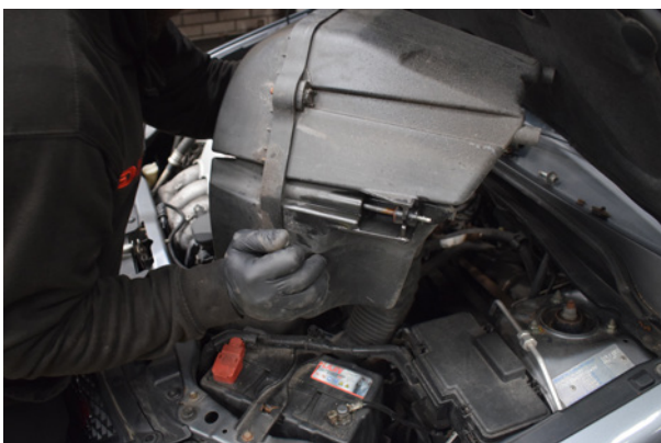
17. The airbox can now be lifted out of the engine bay.
