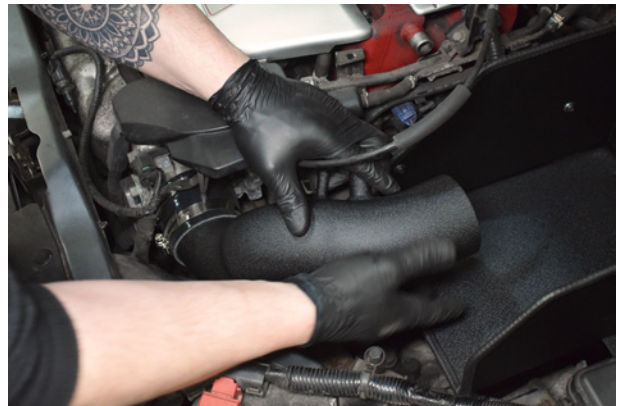
30. Slide the Direnza intake pipe into the silicone.
