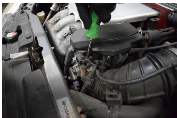
3. Undo the jubilee securing the intake pipe to the throttle body.
