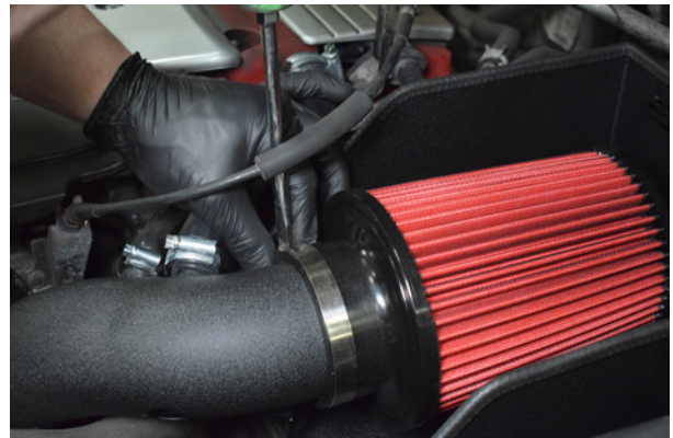
43. Tighten the jubilee to secure the filter to the intake pipe.
