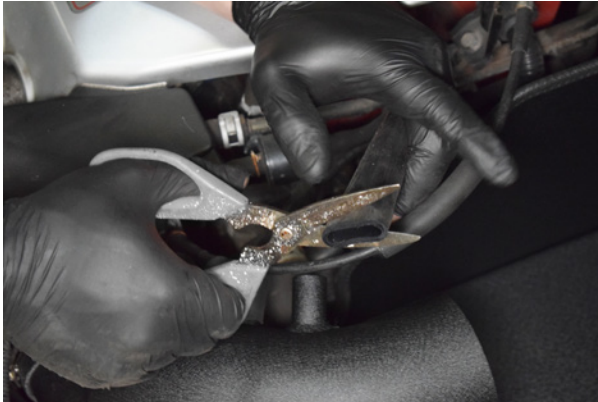
37. The breather pipes may require trimming.
