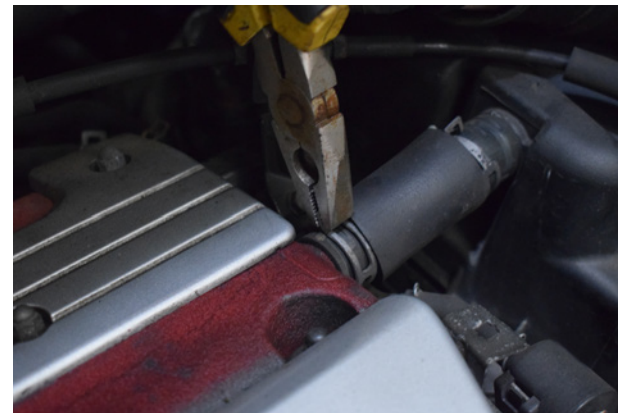
10. Use pliers to squeeze the breather hose clips together and remove the pipe.
