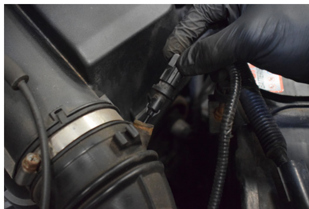
4. Remove the intake temperature sensor.
