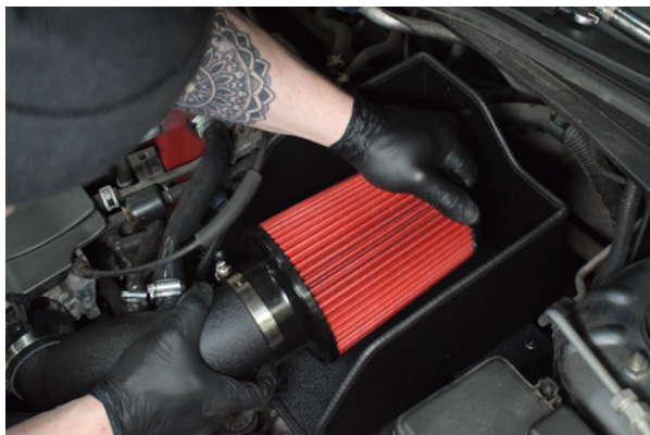
42. Place the air filter onto the end of the intake pipe.
