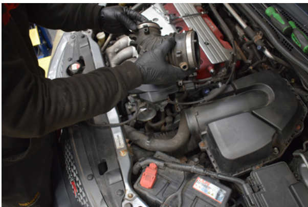
15. You can now remove the intake pipe.
