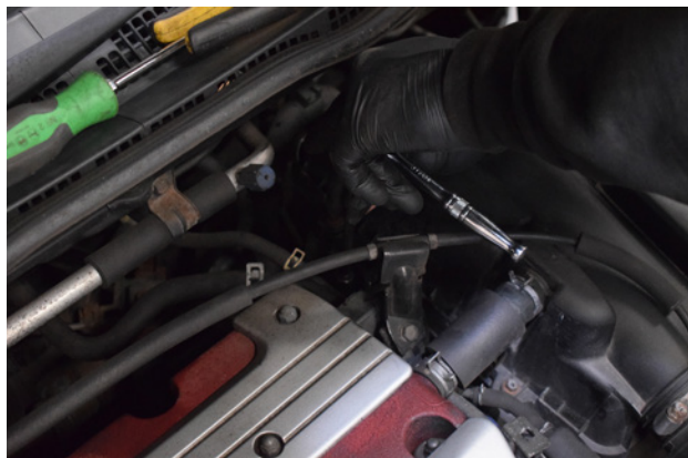
7. The second bolt is located towards the back of the air box.
