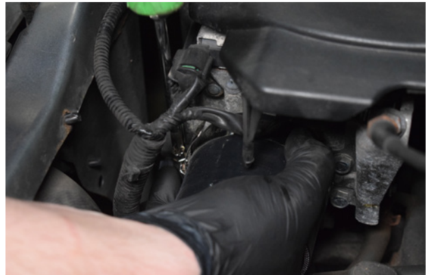
28. Tighten the jubilee to secure the silicone to the throttle body.
