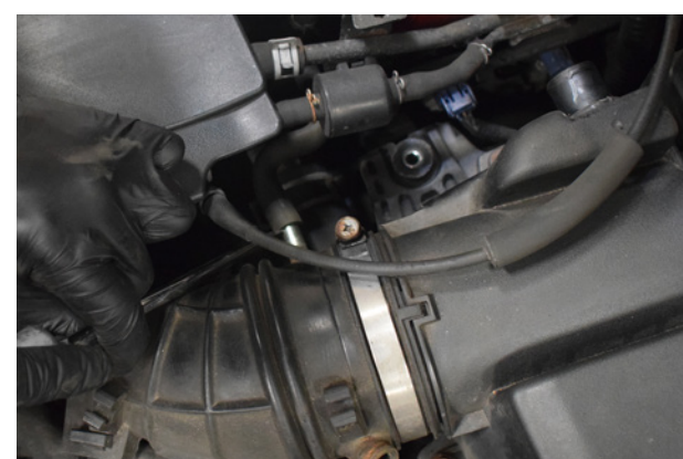
12. Remove the smaller breather pipe.
