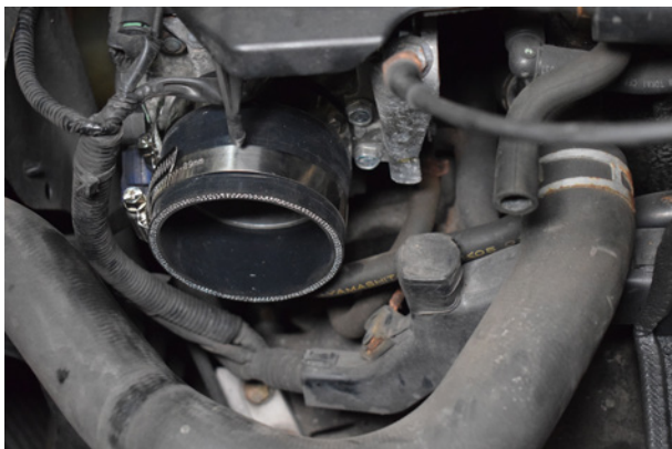
29. Place a second jubilee over the silicone, this will be used to secure the silicone to the intake pipe.
