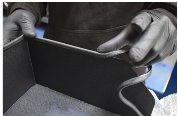
18. Install the edging trim around the edge of the Direnza heat shield.
