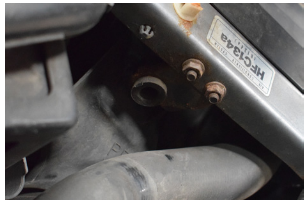
16. Before removing the air box, remove the nut located just underneath the slam panel.
