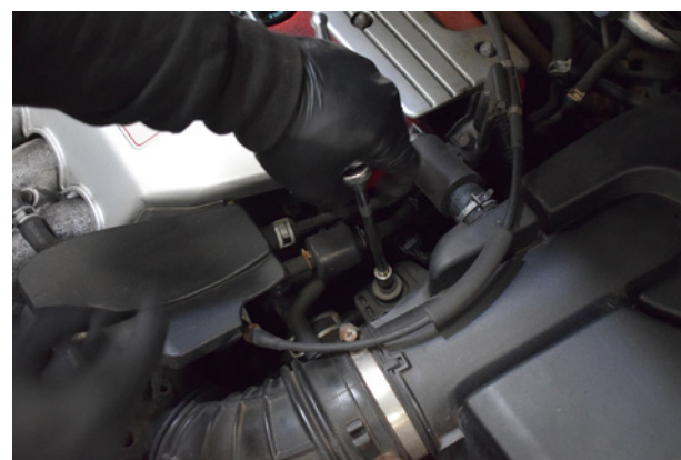
6. Undo one of three bolts securing the airbox to the car.
