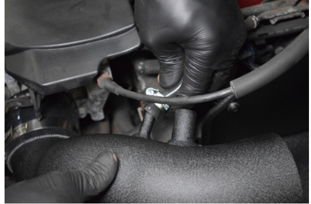
38. Once happy with the length, install the other end of the breather pipe to the small breather outlet on the intake pipe.
