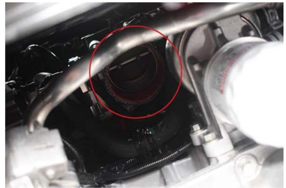
41. Place largest silicone joiner onto the throttle body.
