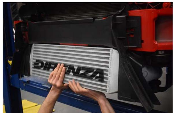
30. Lift MVT intercooler into position, ensuring it is sitting securely on all mounting and guide points.
