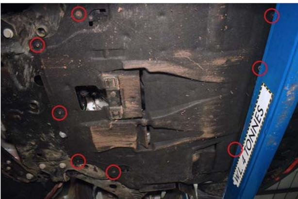
9. Remove 8x Torx on the engine undertray. There are also 2x clips to remove.
