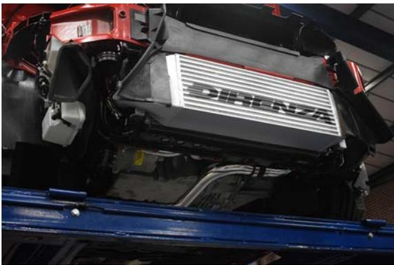
44. Secure all pipes and silicones using supplied clamps each silicone should have two clamps to fix either end of the joiner to the appropriate part.
