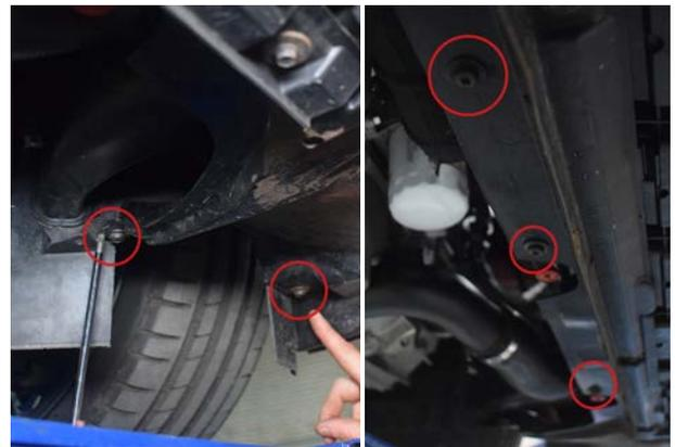
11. Remove 7x screws on front edge of bumper holding on the bumper undertray.
