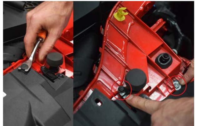
6. Remove 5x screws across top panel & 2x push clips.
