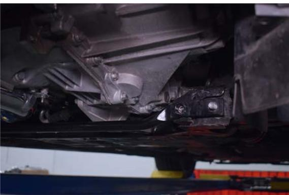
45. Re-install chassis brace by reversing step 17.
