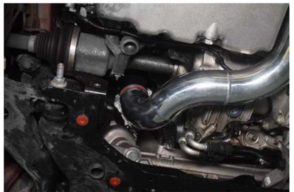
36. Lift boost pipe into position, Secure this pipe to the turbo using supplied clamps.
