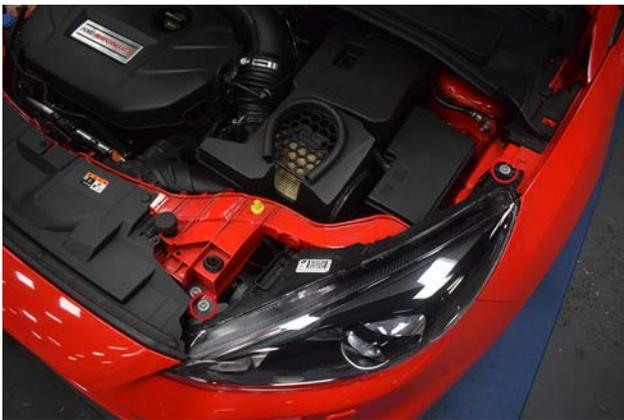
2. Remove the 2x T30 on each headlight unit.
