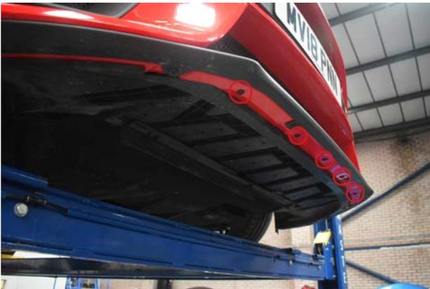
8. Remove 7x plastic screws from the underside of the bumper. You can use the trim tool to help pull these out.
