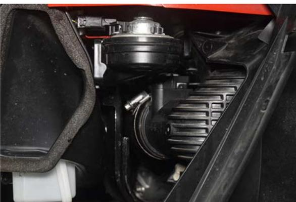
21. Move onto the cold side boost pipe and loosen 2x 7mm jubilee clips.
