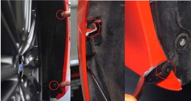
7. Under wheel arch, remove 2x T30 Torx and 2x trim clips. Repeat this on both sides.
