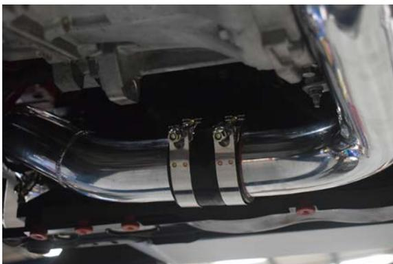
39. Install second hot side connector pipe by sliding it into the two silicone joiners. (1 on the end tank and 1 on the hot side boost pipe).
