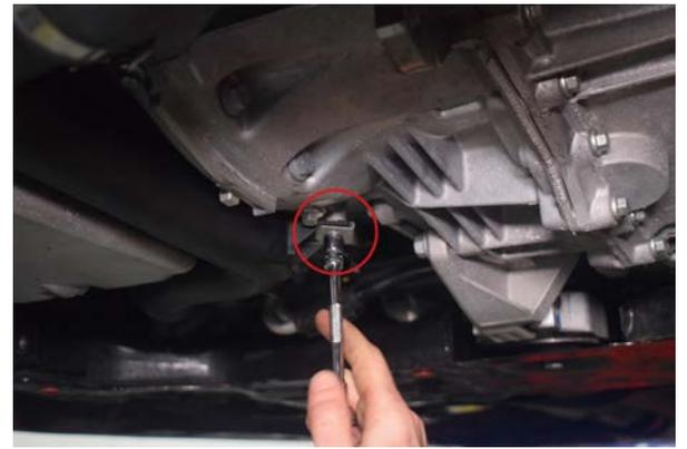
18. Remove 2x 10mm nuts on hot side boost pipe support brackets. We have circled one, follow the pipe to locate the second.
