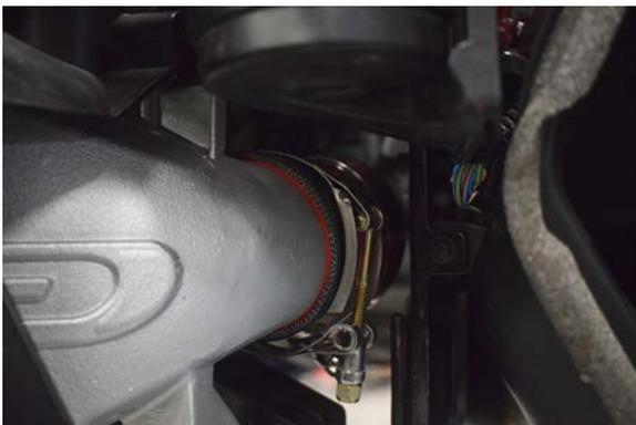
33. Install silicone joiner on the hot side end tank (1 of 3 joiners the same size).
