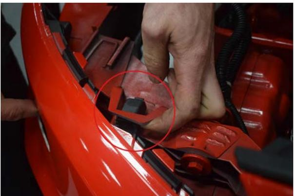
15. Lift clip and push down and rubber stop on the top of bumper, located on the drivers side.
