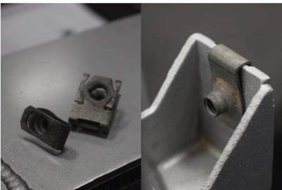
27. Take metal clips from the OEM intercooler and place them onto the equivalent position on the MVT.
