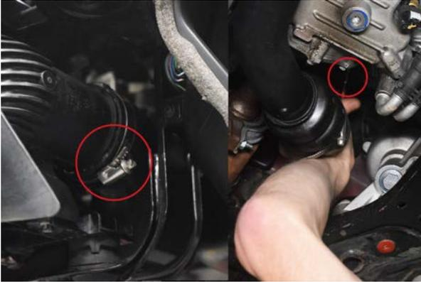
19. Loosen 2x 7mm jubilee clips on hot side boost pipe. One is located near the end tank and one near the turbo.
