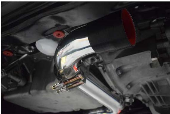
38. Place 2x clamps and silicone joiner onto the other end of the hot side boost pipe.
