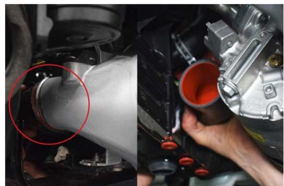
42. Put 90 degree silicone joiner onto the cold side End tank.
