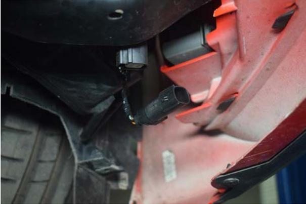
13. From underneath unplug 1x foglight plug. (Located on passenger side).
