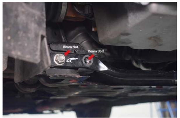
17. From underneath the car, remove 2x 15mm bolt and 2x 18mm nuts on the chassis brace and remove.
