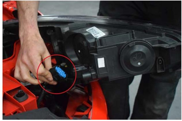
4. Disconnect plug on the back of both headlights and remove the lights.
