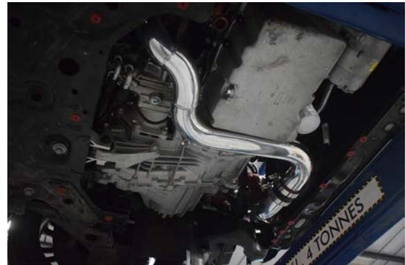
40. Secure all boost pipes and joiners in position by ensuring all clamps used so far are tightened sufficiently.
