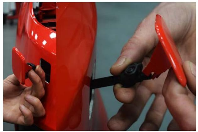
5. Use pick to remove washer jet. Lift and roll upwards to release. Do this on both sides.
