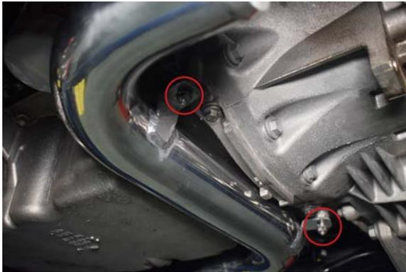
37. Re-install nuts on the hot side boost pipes support brackets.
