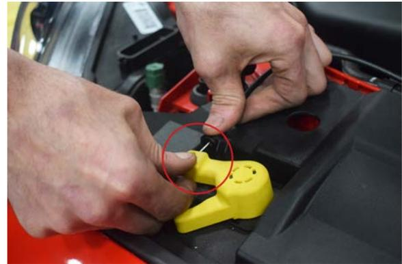
52. Ensure the bonnet safety catch is connected before closing the bonnet!
