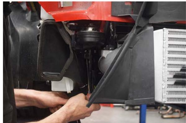
29. You can loosen radiator support brackets (2x 10mm per side) to help fit the MVT.
