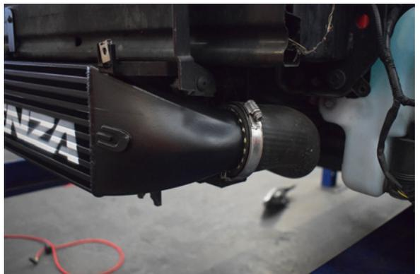
42. Install the intercooler hoses onto the MVT intercooler end tanks.
