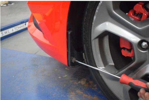
9. To take off the bumper start by removing 4x screws located along the leading edge of the arch liner.
