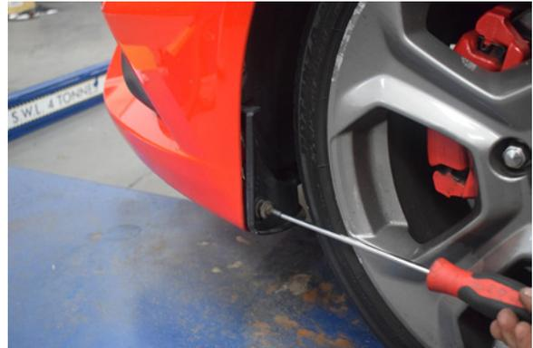
52. Re install 4x screws under inner wheel arch.
