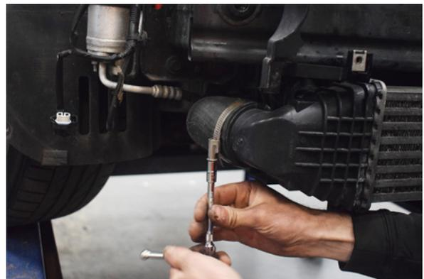
28. Undo 2x jubilee clips on the OEM intercooler using 7mm socket.
