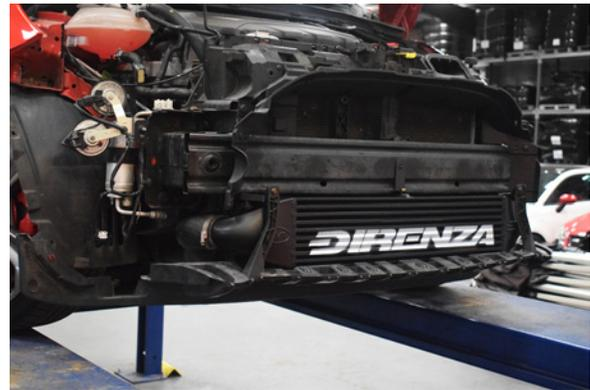
46. The intercooler is now installed and the front of the car can now be rebuilt.
