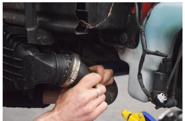
30. The OEM boost hoses can now be pulled off the intercooler.
