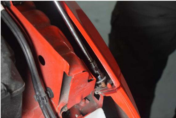
51. Install 3x 10mm inner wing bolts and repeat on the other side.
