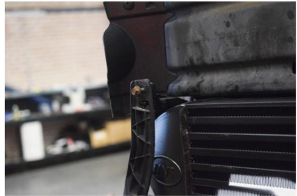
44. Re insert lower shroud trim and install 5x 8mm bolts.
