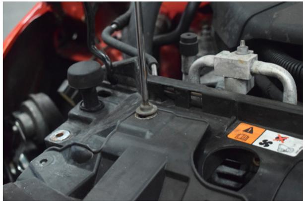
16. Remove 2x T30 screws also located on the slam panel.
