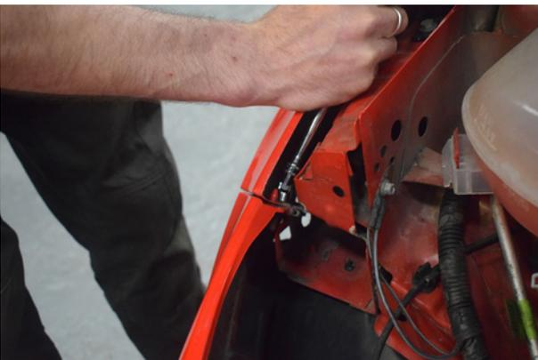
11. Using 10mm socket and extension remove 3x bolts inside the inner wing.
