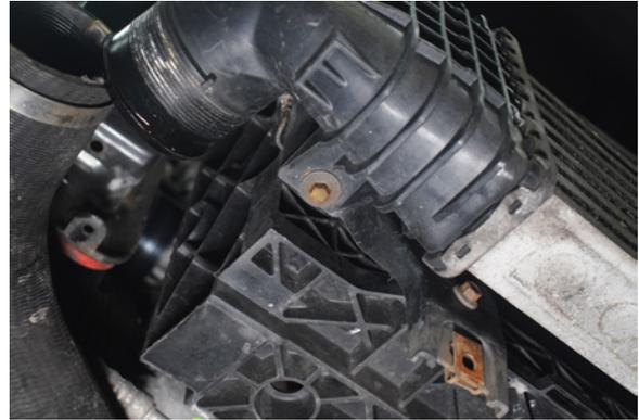
32. From underneath, remove 2x 8mm bolts on the lower intercooler mounting points.
