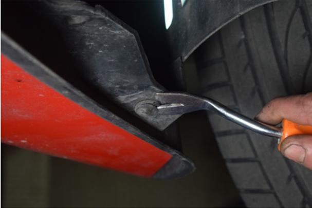
13. Remove plastic clip from under front bumper, one per side.
