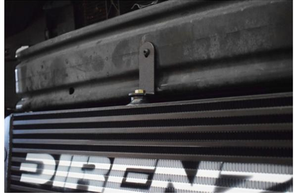
38. Lift the MVT intercooler into position and secure to the mounting bracket using the supplied 13mm bolt.
