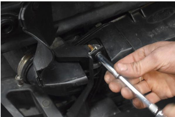
21. You can now remove the intercooler shroud by removing 5x 8mm bolts. 2x at the top and 3x located underneath.
