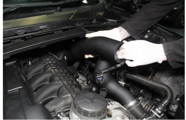
26. Install the rear induction hard pipe.
