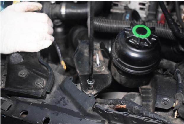
13. Undo 2x 10mm nuts on the second bracket..
