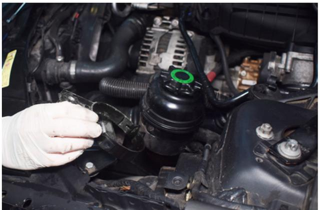
12. Take the reservoir out of the holder and remove the holder from the vehicle.
