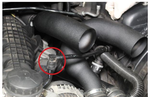
30. Push vacuum pipe back into position ensuring the pipe goes underneath the two hard pipes.
