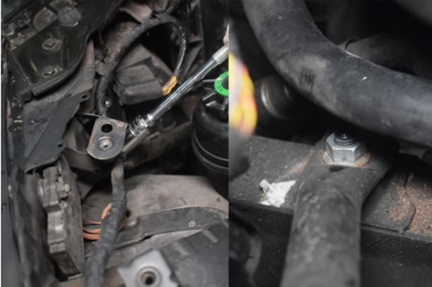
19. Remove the 2x 16mm nuts securing the chassis brace.
