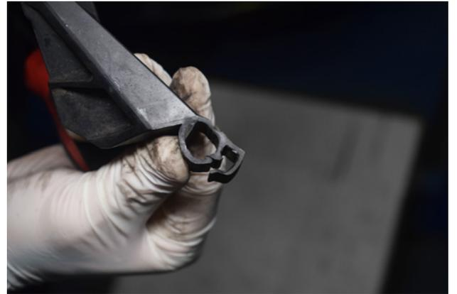
18. Un-clip the bracket from the AC pipe.
