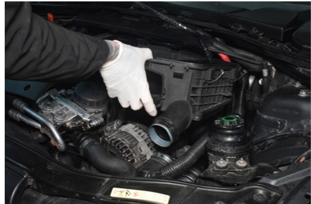
10. Lift up and remove the air box.
