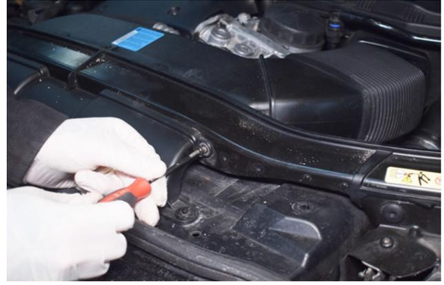
2. Remove 2x T20 securing the OEM air scoop.
