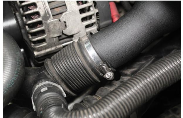
28. Tighten 2x jubilee clips connecting the two hard pipes to the OEM induction pipes.
