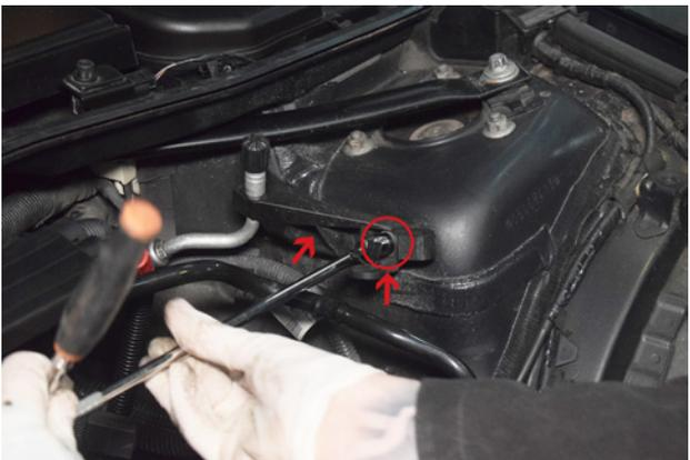
17. Remove the 2x 10mm nuts on the plastic bracket securing the AC pipe.
