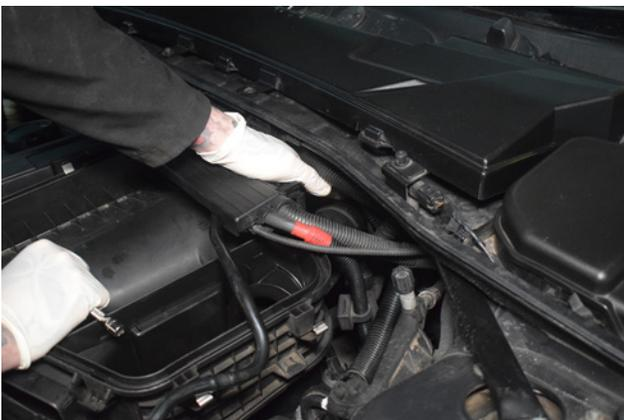
9. Undo the 6mm jubilee on the rear induction feed and remove.
