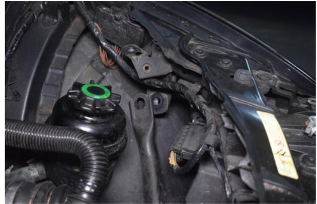
20. Remove the chassis brace.
