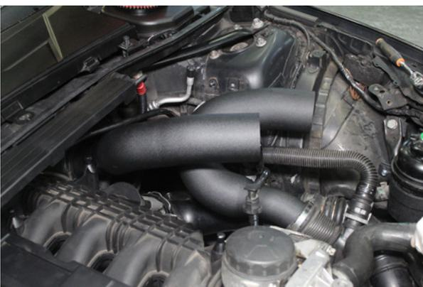
29. Secure the front hard pipe to the passenger side strut tower stud using the nut you removed earlier from the AC bracket.
