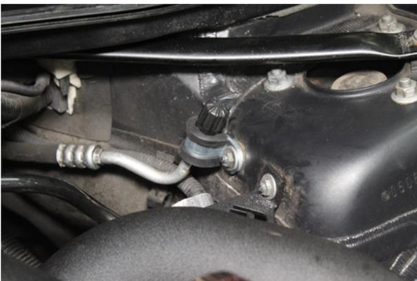
35. Use the second nut from the original AC bracket to secure and fit the new AC pipe and Direnza clamp.
