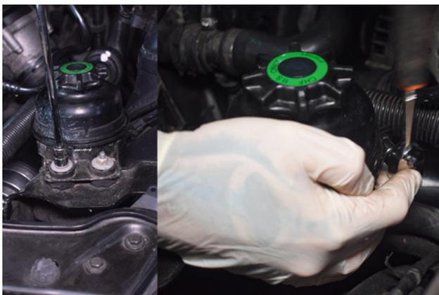
11. Remove the 2x 10mm nuts on the power steering reservoir and the 10mm bolt on the clamp.
