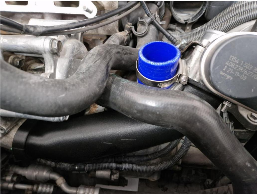
10. Install the bypass hose. Let the hose clamp loose until you secure the intercooler horn.
