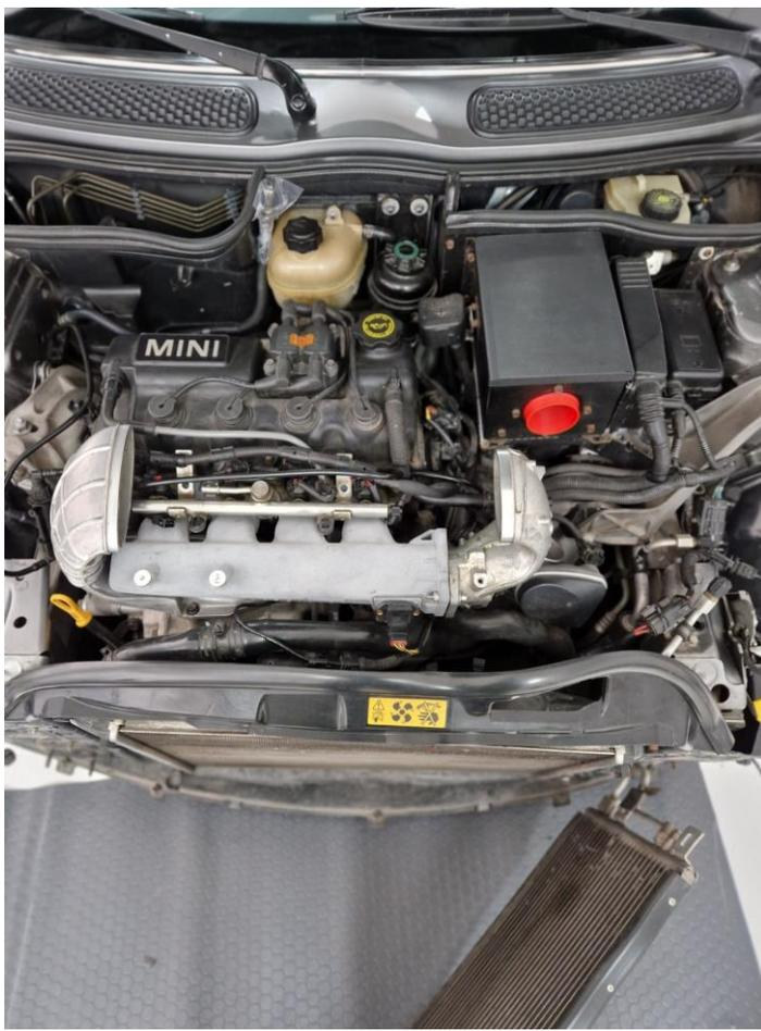
3. Remove the intercooler diverter, the intercooler and the silicone hose that connects the throttle body and the airbox.
