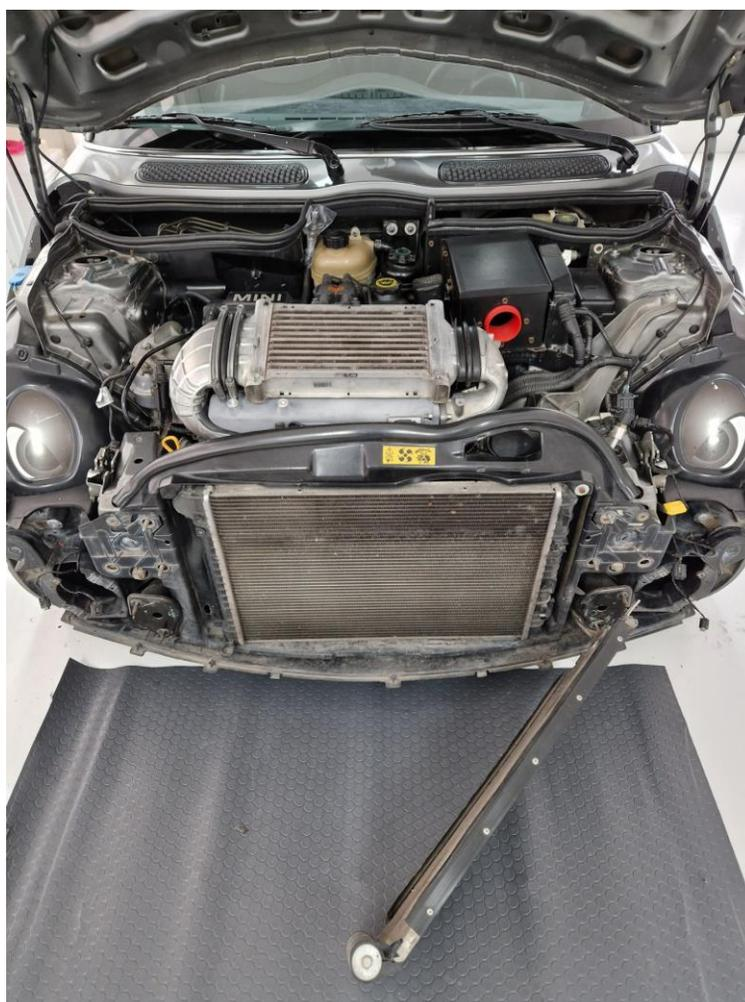
2. Remove the bolts that secure the AC radiator. Carefully put AC radiator aside and pull the plastic shroud that supports the water radiator.
