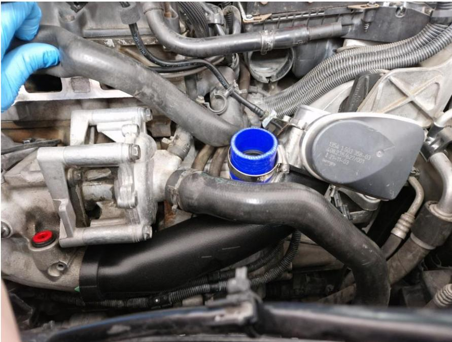
11. Make sure the charge pipe is fitted as in the photos.
