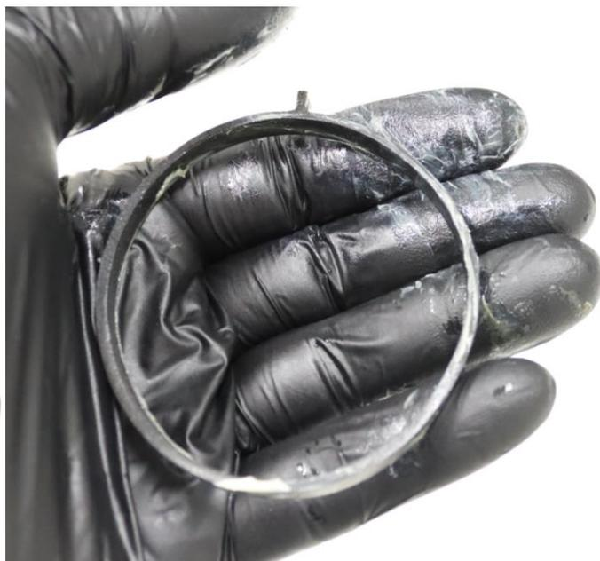
2. In the kit you will find a syringe that contains 5ml of high temp silicone grease. Please apply to all seals before installing them on the manifold. Just spread the silicone grease with your hand all over the seals, as in the photos above.
