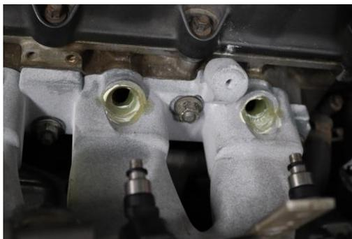
5. Apply a layer of silicone grease in all four injectors holes.
