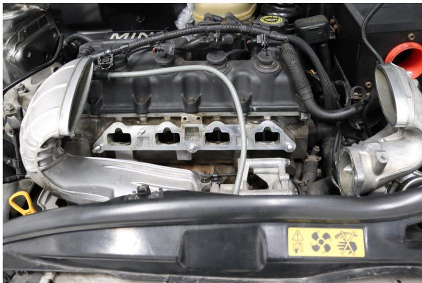
1. Disconnect the battery, remove the intercooler and original intake manifold.
